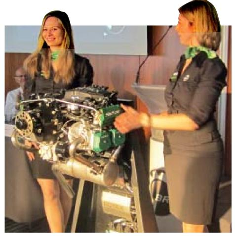
three years, with 10,000 hours of running on the test bench and 700 in the air, and the promise is for lower CO2 emissions and greater fuel economy – the company quoting up to a 21% reduction over the carburetted engine when cruising at 5,000ft. To maintain redundancy, the engine has two independent ECUs that drive double injectors and double spark plugs for each cylinder.
